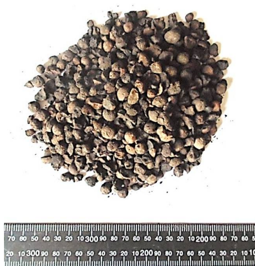
Figure 2. Artificial aggregate Certyd—differentiation of fraction and shape (ruler in mm).
