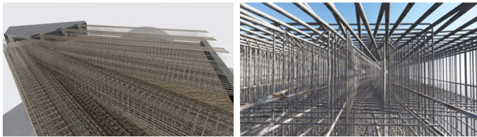
Figure 7. Visualization of reinforcement in the common node of beams BS/1, BS/2 and BS/3.
